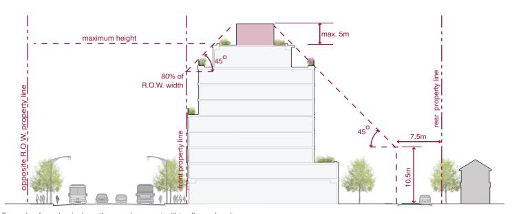
Example of mechanical penthouse placement within all angular planes.
