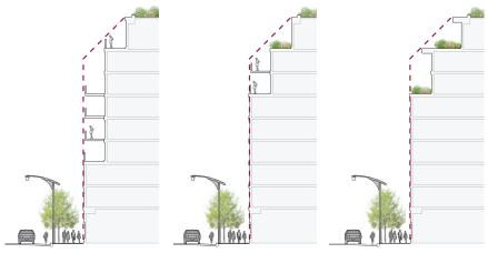
Projection, balconies, railings and overhangs should fit within all angular planes.
