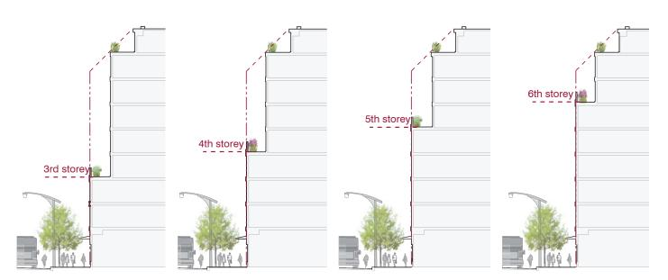
For buildings taller than 23 metres, an additional step-back may be required. The location of this step-back is flexible. The above example illustrates a 9 storey building on a 30 metre R.O.W. which integrates step-backs in accordance with Performance Standard 4A: Front Façade: Angular Plan and an additional Pedestrian Perception step-back.
