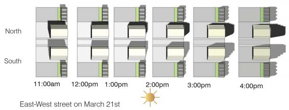
Shadow Testing of Performance Standard 5B (angular plane from 10.5 metres above setback)
