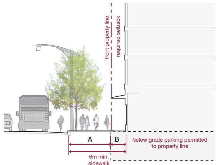
Example of minimum sidewalk width on right-of-ways greater than 30m.
