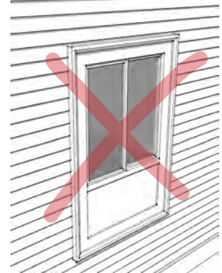
Replacement windows shall be the same style as the original window and shall be the same size as the original window unless the window frame and trim is resized.
