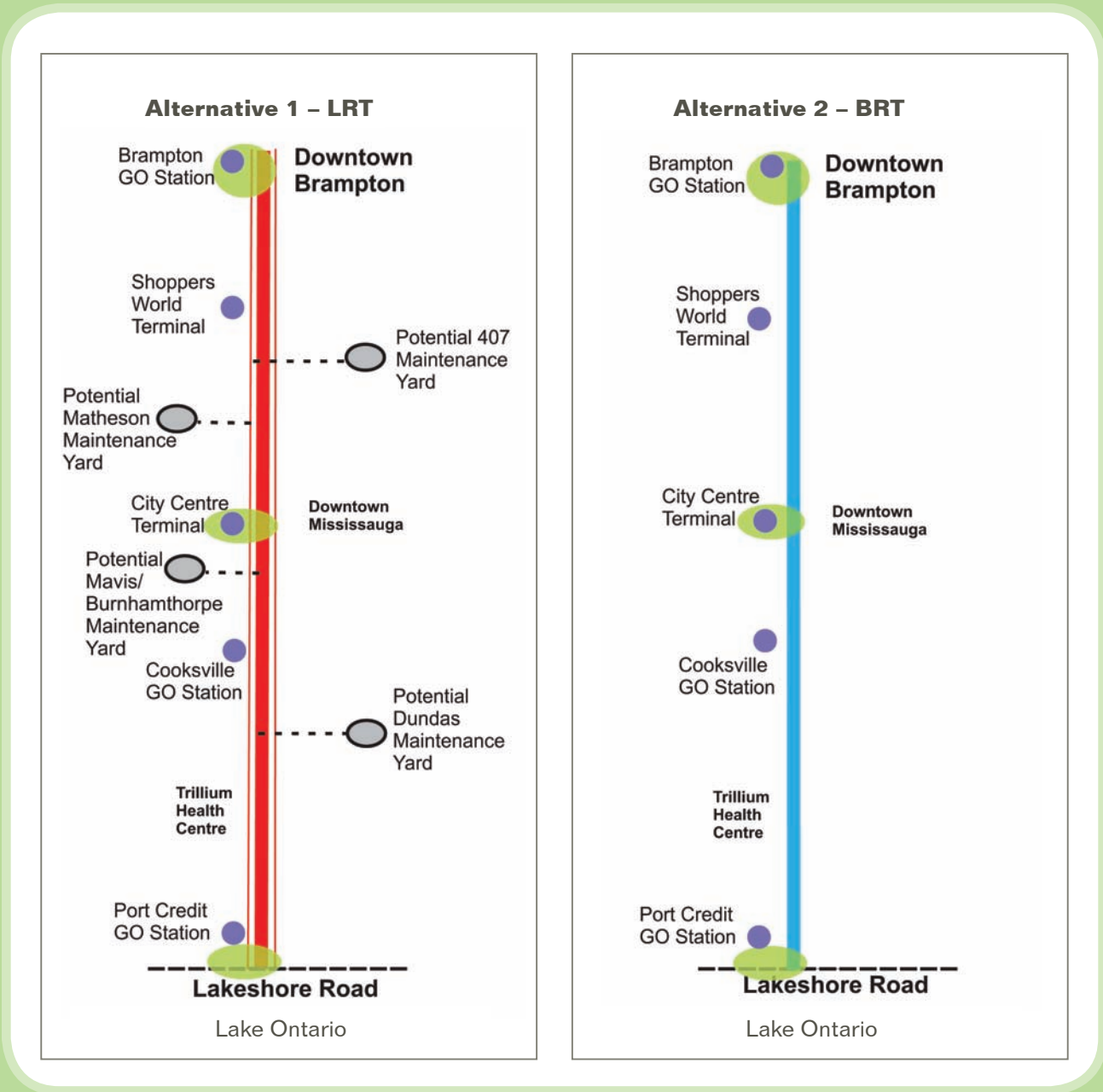
Figure ES.1: Corridor Rapid Transit Alternatives
