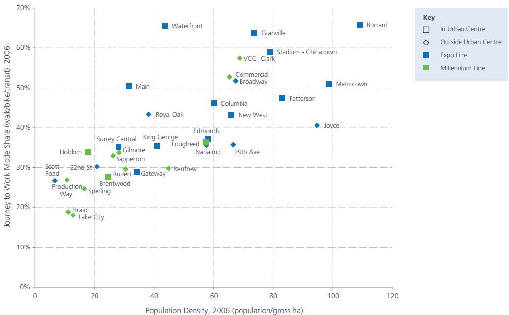
Population Density versus Journey to Work Mode Share (walk/bike/transit) for People Living Within 800 m of a Rapid Transit Station, 2006
