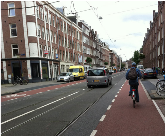
1.5 m bike lane integrated with vehicular/on-street parking lane
