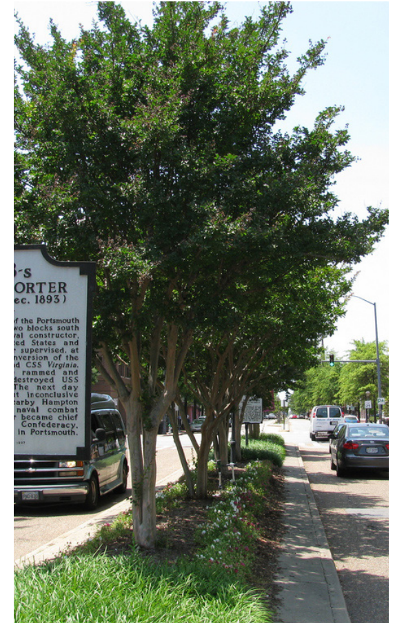
Medians can provide shade, facilitate crossings or buffer lanes of opposing traffic
