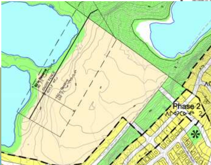
Snow fencing and snow accumulation setbacks in a Community Plan, Hamlet of Rankin Inlet
