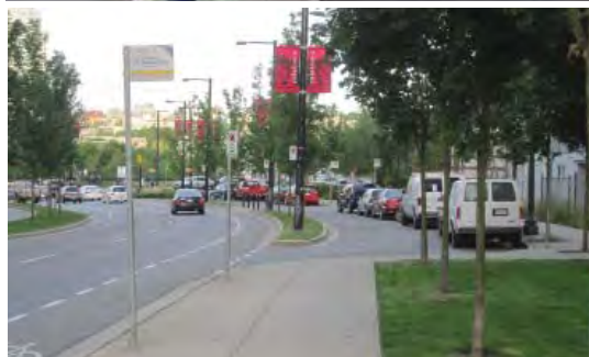
Example of four lane street with median, two slip-lanes, and on-street parking
