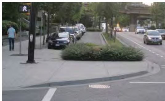
Example of a four-lane street with median and one slip-lane with back-in diagonal parking
